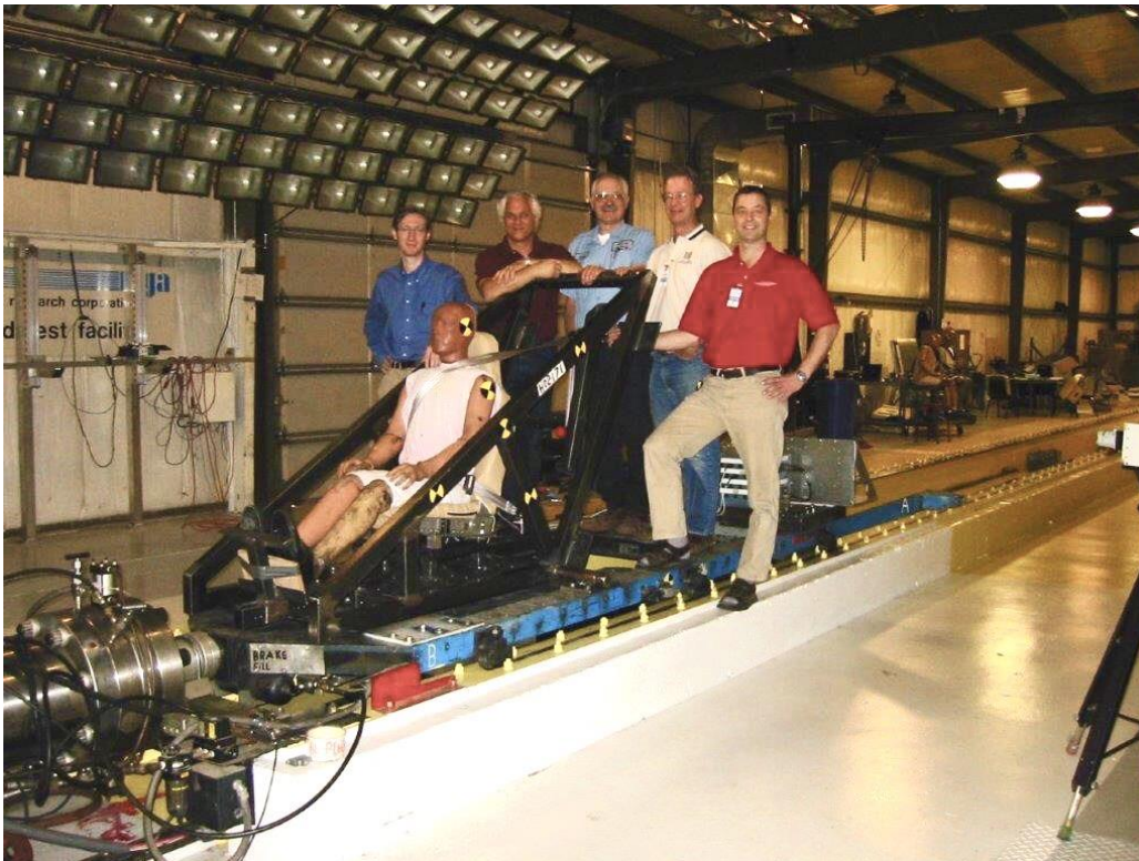
Crash testing at MGA laboratories, the first, and still only, patented, certified crashworthy aircraft seat with no moving, or crushable components able to protect from secondary and even tertiary hits.
