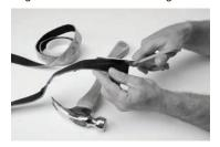
5. Next we will apply the 1" wide clear protective tape in a spiral fashion in the opposite direction of the shock-absorbing tape. There will be no need to cut the ends of this layer at an angle as an overlap is recommended. Begin the wrap by overlapping the the first wrap over itself. Then continue the spiral, allowing the edge of the clear tape to overlap slightly as you go. Finish off this layer with a final overlap of clear tape and cut the excess material away.
