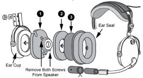
Testing shows the HushKit outperforms ANR headsets in the 700-7000Hz range where hearing loss occurs. Four die-cut, visco-elastic foam layers fill the voids of the ear cups and decouple the speakers from the housing. The result is reduced noise and improved intelligibility. In a noisy cockpit, you can actually turn down your radio's volume. It's not that you can't hear your radio, it's that you can't understand what's being said in the voice frequency range.
